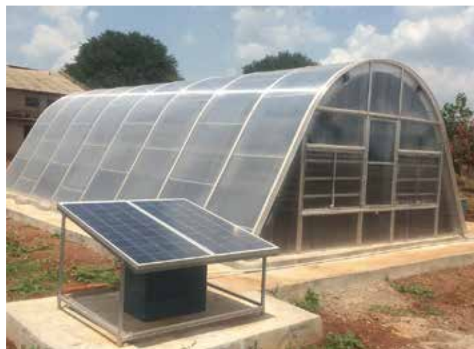
Hybrid solar dryer with solar collector and an artificial heating chamber for drying in the absence of sunlight ( left ); greenhouse solar dryer for high volume and quality chili drying ( right ).
