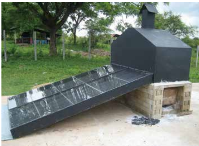
Hybrid solar dryer with solar collector and an artificial heating chamber for drying in the absence of sunlight ( left ); greenhouse solar dryer for high volume and quality chili drying ( right ).
