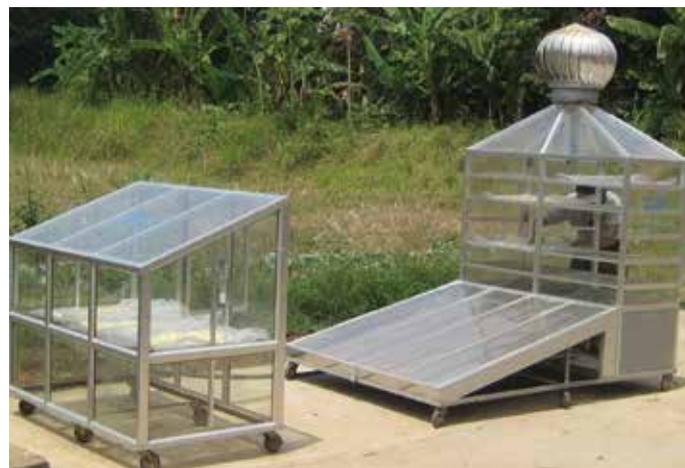
Solar heat collector-equipped dryer and cabinet solar dryer for drying chili peppers (left) and cabbage (right).
