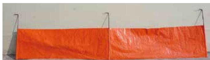
Nylon sheet with inserted iron bars
